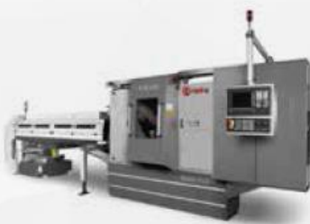
CNC shaft turning m/c
